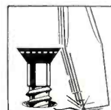
Slipping driver scars surface or injures workman
