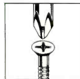
The tapered driver fits the Phillips recess
