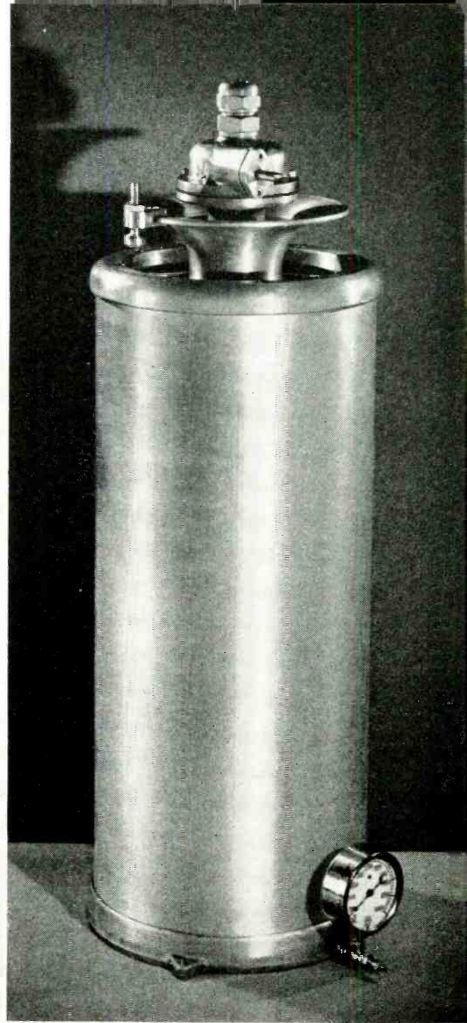
Lapp variable condenser Y150V15 100 amp., 15 KV (carrier RMS, 100% modulation) Capacitance 600-1500 mmf. External dimensions: Height, 34", diameter, 11"
