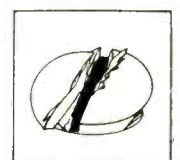
Slotted screw's head may split when tightening
